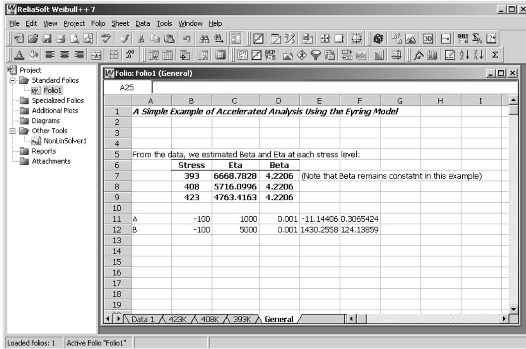
To aid in the process of calculating eta at different stress levels, the parameters A and B will be defined as named variables within the spreadsheet. This allows you to reference these values in a formula without having to input the actual value.
