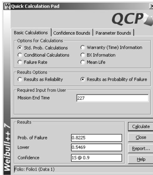
The QCP returns a result of  $Q(T) = 0.8225 \cong 82\%$ . This agrees with the result found using the plot. However, using the QCP is more accurate and easier to use.
