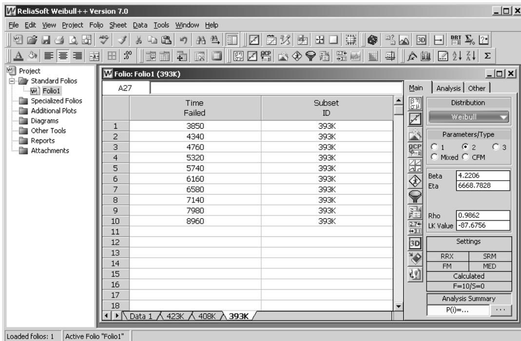
You will notice that three new data sheets labeled 423K, 408K and 393K will appear in the Folio. Each data sheet contains the data that has been extracted for the specified Subset ID (*i.e.* stress level). You can click each tab to view the new data sheets. Notice that the parameters have already been calculated for each stress level.
