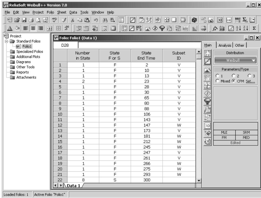
When the CFM option is selected and you click Calculate, the Competing Failure Modes Select Subsets window will appear. This allows you to identify the competing failure modes, based on Subset ID. Note that you can also open this window by clicking the **Set...** link to the right of the CFM option.
