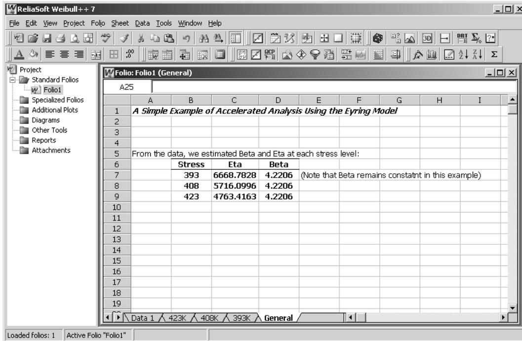
The Non-Linear Equation Fit Solver can be used to estimate the parameters of the Eyring model.<sup>8</sup>
