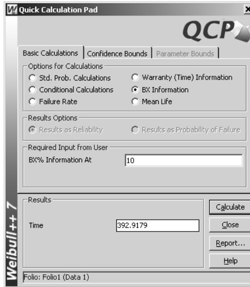
Using the Degradation Analysis utility and the QCP, the B10 life is calculated to be 392,918 cycles.
