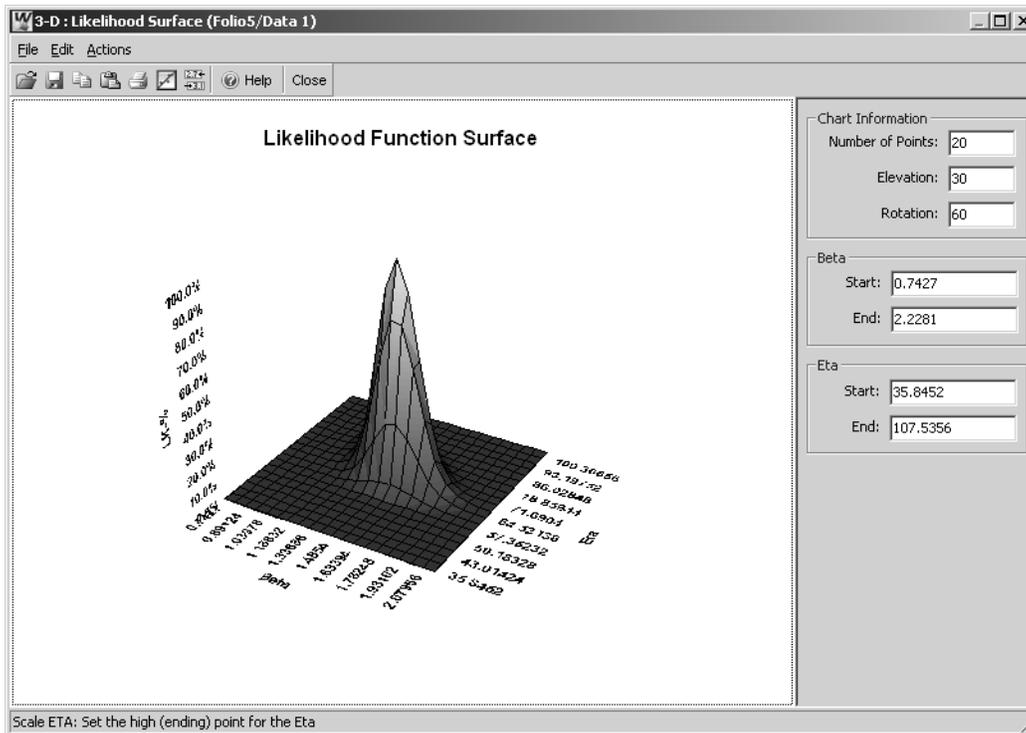
To rotate the plot, click the plot then press the **Ctrl** key while holding down the left mouse button and moving the mouse. Note that the peak of the surface is at the center of the beta-eta plane.
