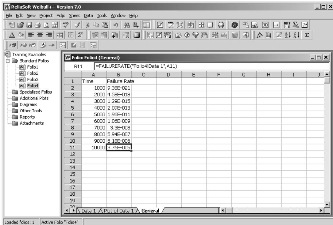
The table that you have created displays the failure rate for each time in column A, based on the analysis in the associated data sheet.
