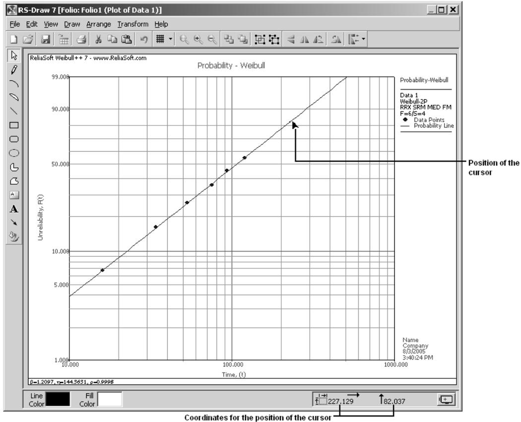
The value of the y-coordinate from the Position Indicator, the unreliability  $Q(T)$ , is such that  $Q(T) \cong 82\%$ . Therefore, a good estimate of the probability of failure (unreliability) at 227 hr is 82%. The reliability is then:
