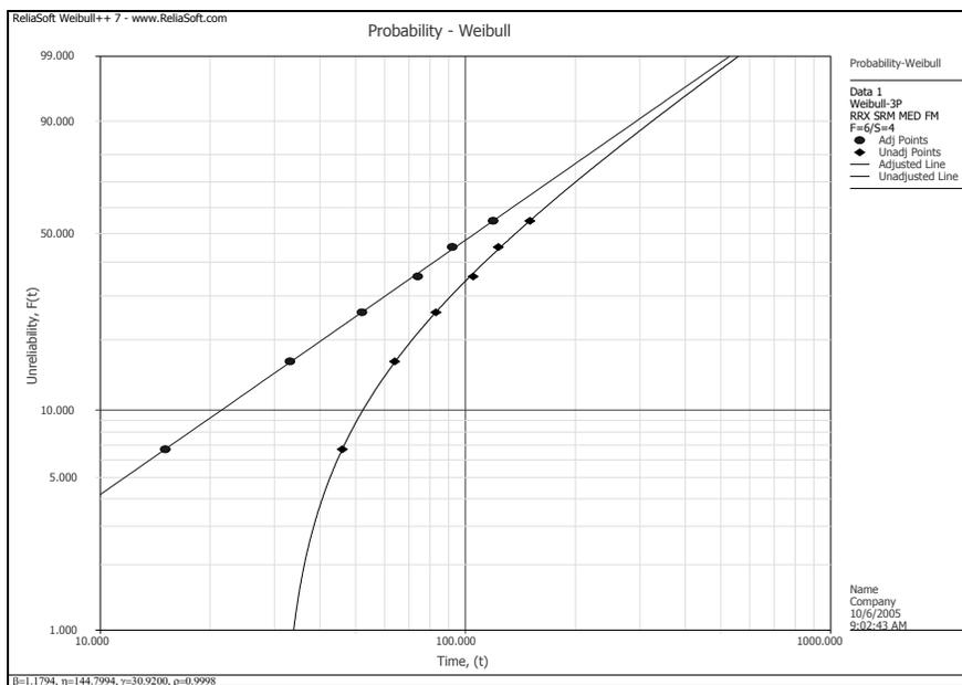
Note that the original data points, plotted along the curved line, were adjusted by  $\gamma = 30.92$  hr to yield the straight line. Also note that the x-axis for the plot is  $T - \gamma$ . Therefore, to obtain the time ( $T$ ) required for a given unreliability level using the straight line, you must add the value of  $\gamma$  to the x-axis value found at ( $T - \gamma$ ). Alternatively, you can read the results from the unadjusted line.
