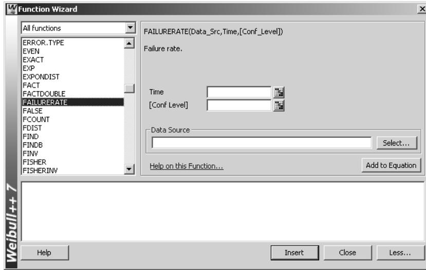
The inputs required for the selected function are displayed on the right side of the window. The text box at the bottom of the window allows you to build the function that will be inserted into the spreadsheet.
