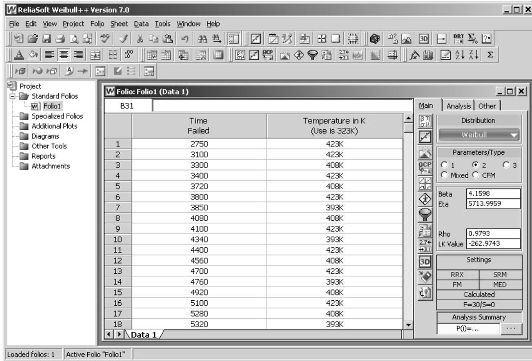
The Batch Auto Run feature allows you to break down the original data set into three different data sets based on the different operating temperatures. The Batch Auto Run uses the Subset IDs to extract the data.<sup>7</sup>
