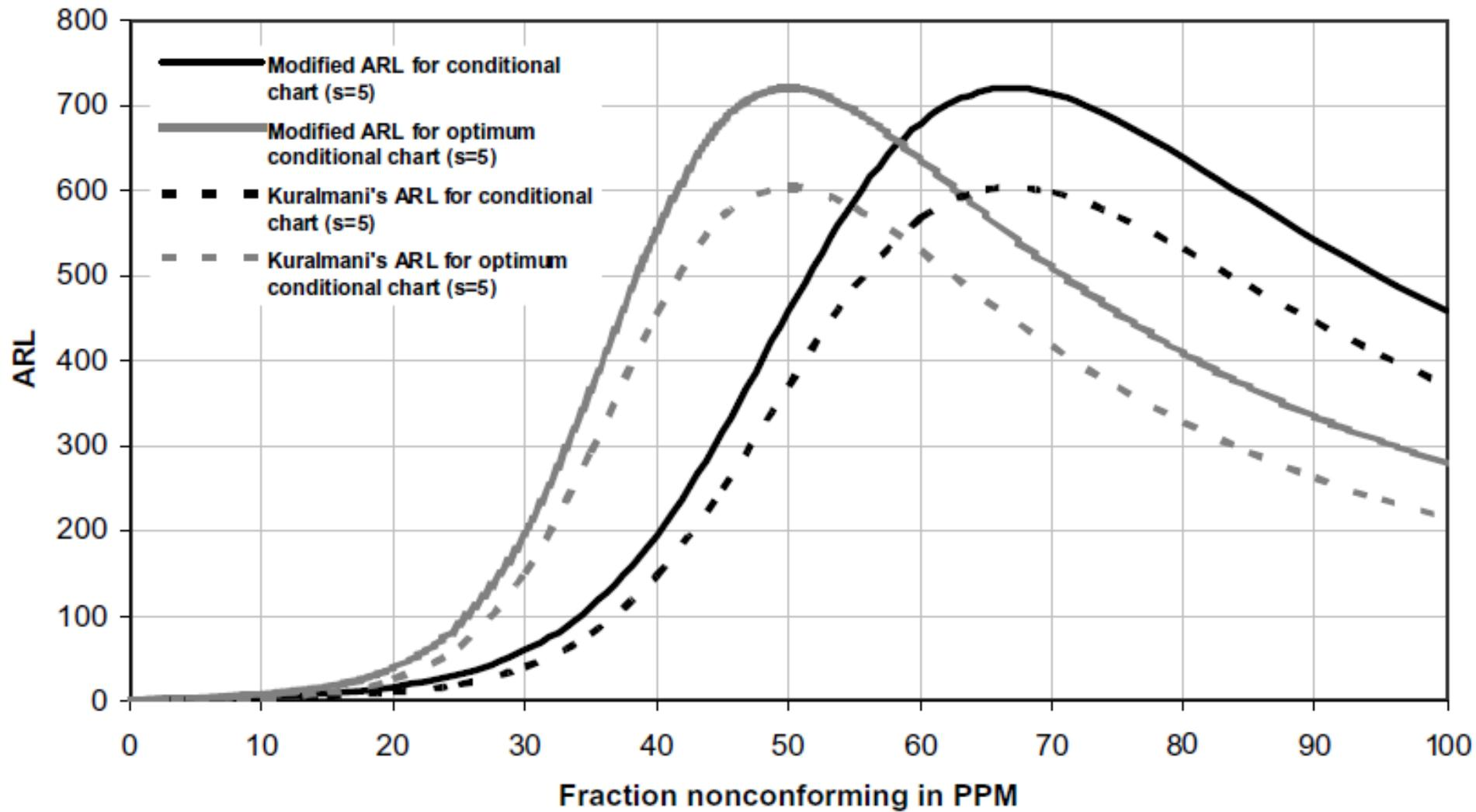
Fig. 2. ARL curves for  $s = 5$  and  $p = 50$  ppm.
