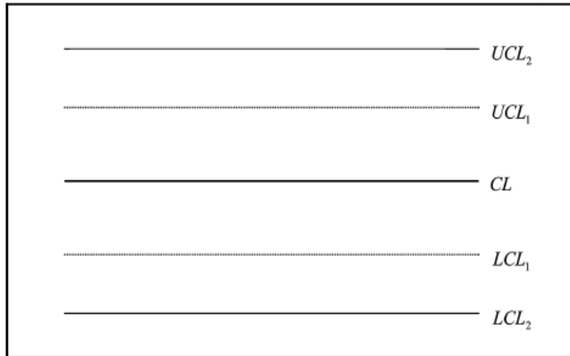
Figure 1. Control limits for a Shewhart \bar{X} chart incorporating either the improved two-of-two or improved two-of-three rule.
